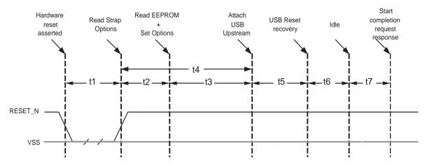
Figure 4.4 Reset\_N Timing for EEPROM Mode
